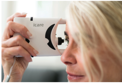
Figure 3. The iCare Home tonometer allows patients to measure IOP at home.
