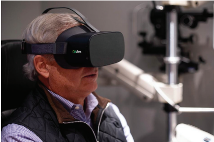
Figure 6. The VisuALL VR visual field perimeter was designed for standardized and mobile assessment of the visual field.
